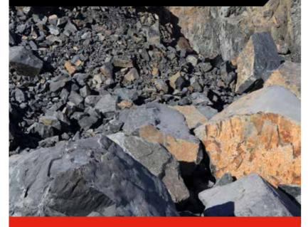
Optimal blast fragmentation saves on overall energy consumption and improves downstream plant performance.
